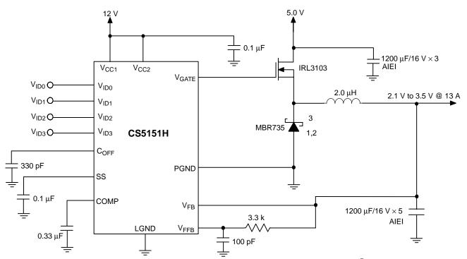
Figure 1. Application Diagram, Switching Power Supply for Core Logic – Pentium<sup>®</sup> Processor with MMX Technology
