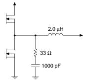
Figure 18. Filter Components
