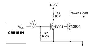
Figure 15. Implementing Power Good with the CS5151H
