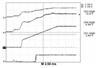
Trace 3 – 12 V Input (V<sub>CC1</sub>) and (V<sub>CC2</sub>) (10 V/div.) Trace 4– 5.0 V Input (2.0 V/div.) Trace 1– Regulator Output Voltage (1.0 V/div.) Trace 2– Power Good Signal (2.0 V/div.)
