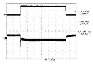
Trace 1– Regulator Output Voltage (1.0 V/div.) Trace 2– Regulator Output Voltage (20 V/div.)
