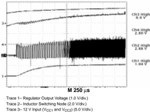
Trace 3- 12 V liput (VCC1 and VCC2) (5.0 V/div.) Trace 4- 5.0 V liput (1.0 V/div.) Figure 4. CS5151H Demonstration Board Startup in
