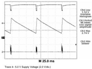
Trace 3– Soft Start Timing Capacitor (1.0 V/div.) Trace 2– Inductor Switching Node (2.0 V/div.)
